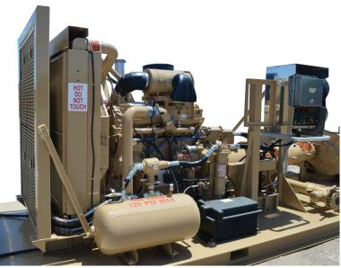
The unit is a 630 horsepower triplex skid mounted pumping unit that is equipped to operate at the work site independent of other equipment. The unit is fabricated on three 10" x 35 lbs. I-Beam. Equipment consist of one diesel engine, automatic transmission, triplex pump, and a centrifugal pump.
