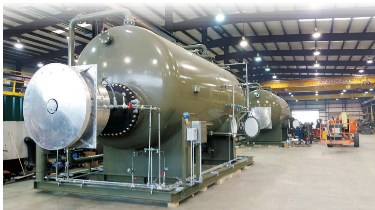
Horizontal Heater Treater
