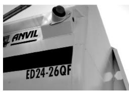
Radius Flanged Front Bulkhead: stronger built welds away from the corner reduces stress concentration in critical areas.
