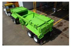
Dual Hydraulic operated sliding doors with complete cover enclosure makes this the ideal drill cutting hauling trailer.
