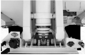
**Inverted Trunnion Cylinder:** reduces maintenance on cylinder wiper seals.
