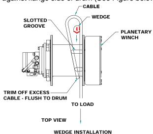
Pull on cable to securely "cinch" cable and wedge into slotted
