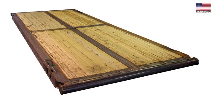
The average life of a Rig Mat is 10 years but constructed soundly it can stay active for up to 20 years. Our  $8' \times 20'$  and  $8' \times 40'$  Rig Mats consist of independent wood sections made up of rough cut  $2'' \times 6''$  treated pine nailed together for superior rigidity. Our Rig Mats are made with  $6 \times 15$  beam cross members unlike other mats that are made with flat bar cross members.
