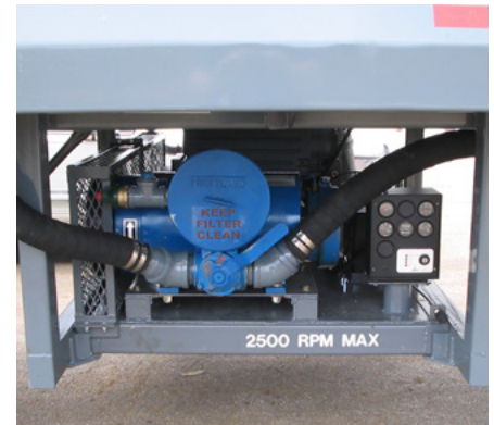
Optional Underbelly Self Contained Pump System
