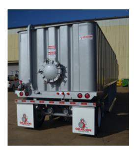
Floor: 1/4 pl, round bottom tub with full length center channels
