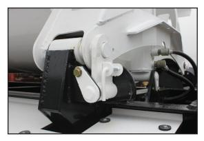
Main hinge rollers, steel housing bushing with a UHMW inner bushing, mounted in structural seats carrying the loads directly in to the coupler or suspension areas. Quick tub dump directional changes without extra pins or plates to carry around.
