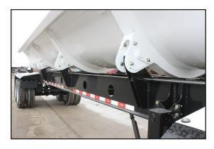
Middle idler hinge rollers, steel housing bushing with a UHMW inner bushing, to ensure smooth and continuous rotational dumping.
