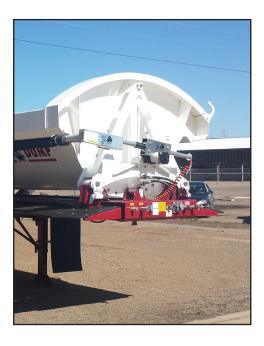
'Patented 'A' Frame Dumping Structure' ensuring that the tub dumping is acting on the bottom of the tub, therefore avoiding the cracking upper tub corners that are prevalent in the industry
